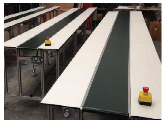
BHH Head Drive Non Wandering Drive Type Conveyor
