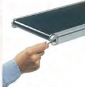
Fine tracking adjustment is done at the tail section.
