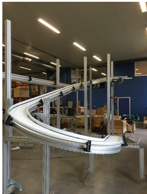
Carryline Helical conveyor, in-decline in curves
